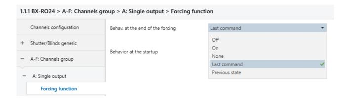
This parameter specifies the behaviour of the switch at the end of the forcing command. It is possible to choose between various options. If "Last command" is chosen, after the forcing is disabled, the last command from the bus will be implemented for that channel. While, the "Previous state" option will restore the switch state before the forcing command.
