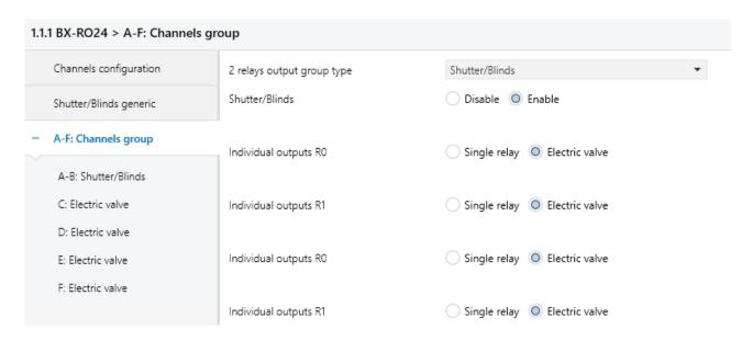
In this case Shutter/Blinds is a 2-outputs function, while electric valves are 1-output function. Thus, channels dedicated to the Shutter/Blinds function are placed in the
