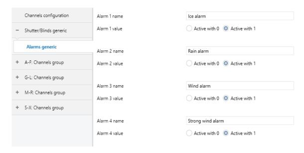
Four different alarm levels are available with the possibility of managing them individually. This function was created to prevent damage to the load connected to the individual device channel (e.g. roller blinds, Venetian blinds, shutters); alarm signals are normally a consequence of atmospheric events detected and sent on the bus by other devices connected to the system.
