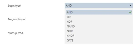
The GATE operation passes the result of the previous operations only if the current logic input is active. If the current logic input is not active, the last result is maintained regardless the actual state of the logic inputs.
