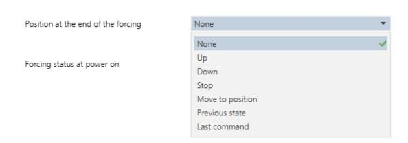
This parameter specifies the behaviour of the channel at the end of the forcing command.
