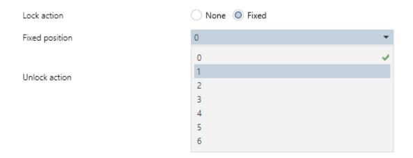
Where 0 means all outputs deactivated, 1 means first output active, 2 means second output active and so on.
